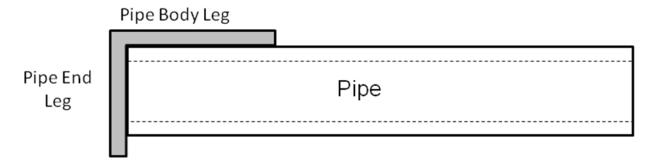
Figure 3—Reference When Using a Fixed Square Measurement
