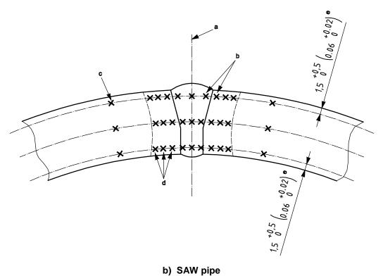
Figure H.1—Location of Hardness Tests
