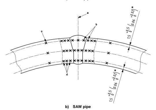
Figure N.1—Location of Hardness Tests
